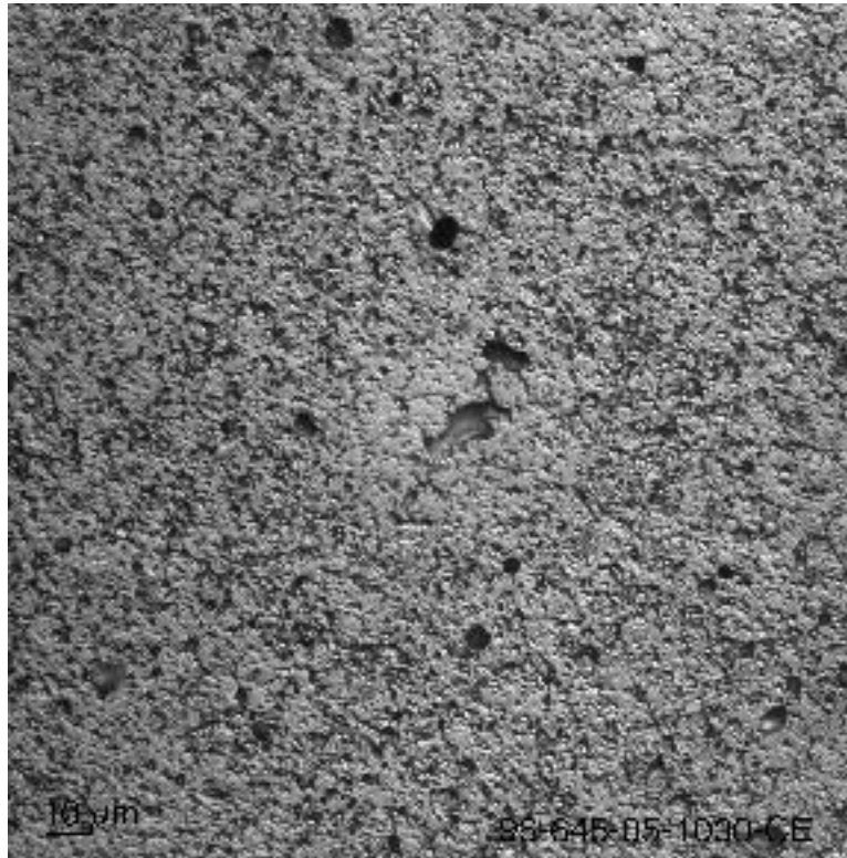
Fig. 38. Optical micrograph of EMOX fuel (magnification: 1000x).
